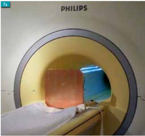
Figure 7. Experimental set up with a square patch antenna.
